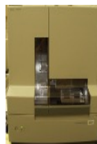
ABI 3100 DNA Analyzer, 16 capillary array.
