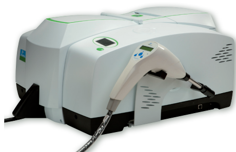
Frontier NIR system with fiber optic sampling: Raw materials identification
