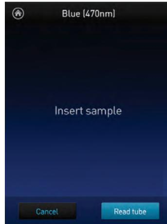
4. For Blue excitation, the Qubit<sup>®</sup> 3.0 Fluorometer displays both the green emission and the far red emission of your sample. For Red excitation, the Qubit<sup>®</sup> 3.0 Fluorometer displays only the far red emission of your sample.
