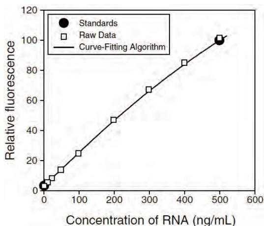
**Figure 1.** The curve-fitting algorithm used to determine concentration in the Qubit<sup>®</sup> RNA assay. Data for other Qubit<sup>®</sup> assays are generated by similar algorithms.
