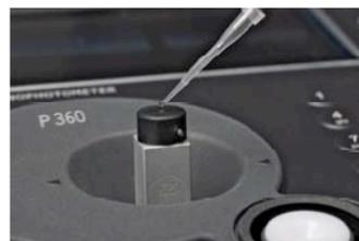
**Step 3** Pipette the appropriate sample volume onto the centre of the measuring window. **Warning!!** Do not overfill the well.
