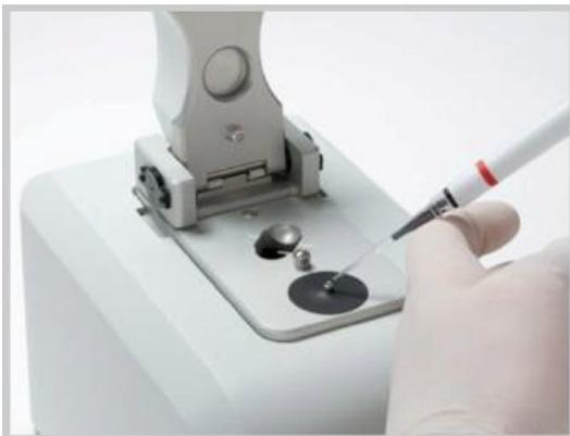
2. Lower the sampling arm and initiate a spectral measurement using the software on the PC. The sample column is automatically drawn between the upper and lower pedestals and the measurement is made.
