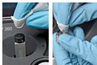
**Step 4** Take the lid off and retrieve the sample with a pipette for further applications if desired. Remove sample residues from the measurement window and the mirror in the lid. Clean the measurement window and mirror in the lid well with a slightly wet fluff-free tissue. Use water, 70% ethanol or isopropanol. Do not use aggressive solvents like strong acids or bases or organic solvents at any time.
