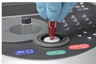
**Step 2** Use the integrated vortexer (P 330 / P 360 only) to mix your sample well to achieve an accurate homogeneity of the sample.
