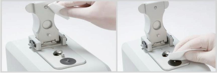
4. Put dry, lint-free laboratory wipe in between pedestal. Close the software.
