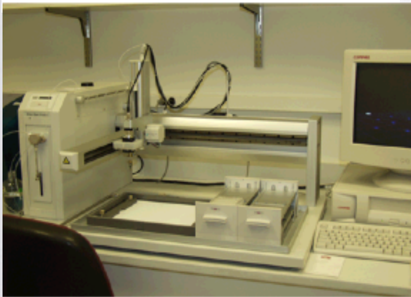
Ettan II 2D gel Proteomics System complemented by a MALDI TOF/TOF(ABI) Model 4800+
