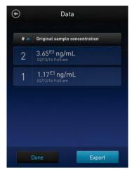
4. To view the sample details, touch the **sample of interest**. A *Data details* screen opens.
