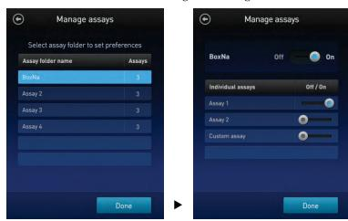
4. To hide all of the assays in the assay folder, swipe the **Assay folder On/Off** switch located to the right of the assay folder name to the **Off** position (to the **left**).
